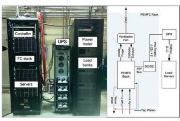
In-Rack Test Unit and System Schematic
