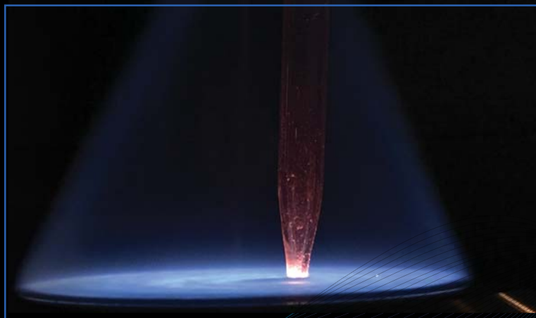
Figure 1. Quartz Microprobe Sampling the Laminar Flat Flame Produced by Premixed Natural Gas, Hydrogen, and Air
