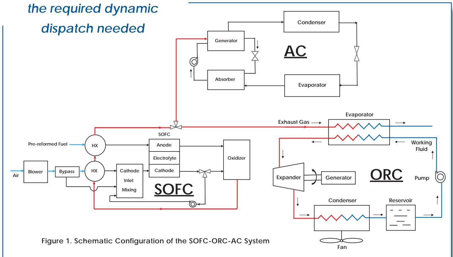
Figure 1. Schematic Configuration of the SOFC-ORC-AC System
