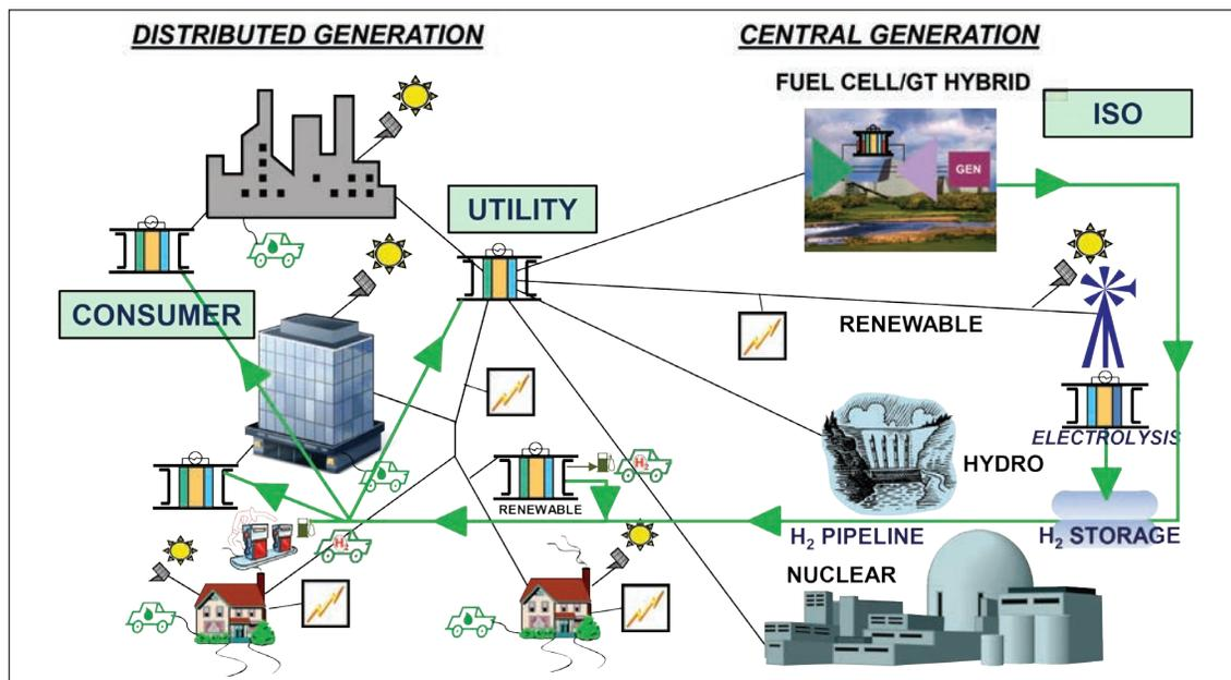
A Schematic Depicting the Elements of the Evolving Electric Grid
